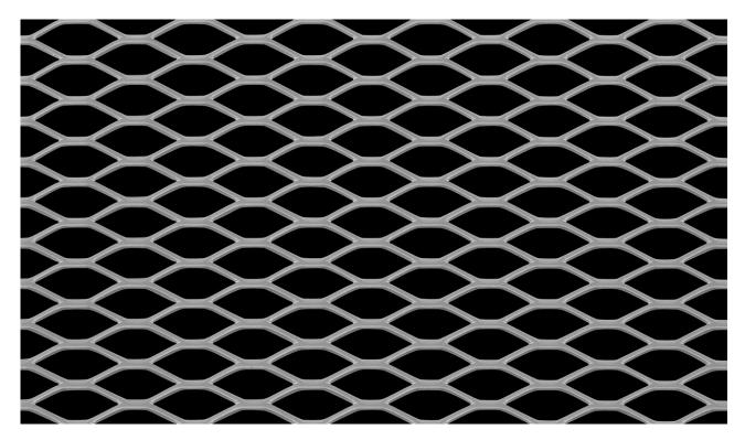
LW Pitch:28.58mmStrand Width:1.65mmSW Pitch:9.52mmThickness:0.90mmWeight:0.85 kg / m2Open Area:65%
